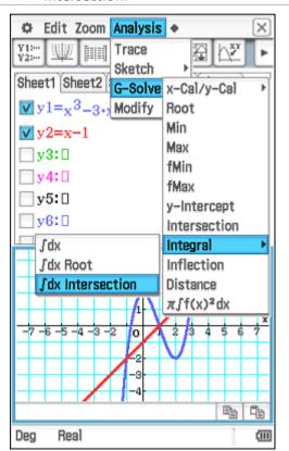
The cursor appears at the left hand most intersection of the functions and the prompt for the Lower bound appears in the bottom right hand corner of the screen.
